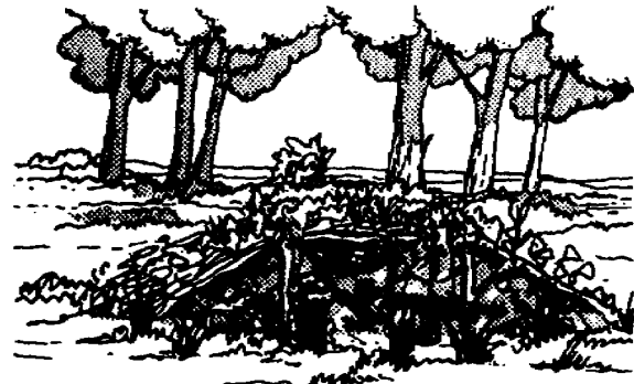
① FOXHOLE WITH CAMOUFLAGE COVER IN PLACE
